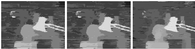
Fig. 5: Experimental results for the Tsukuba dataset [8]. Left, middle: 192 \times 144 , 3-bit FPGA, and numerical disparity result. Right: 384 \times 288 , 4-bit numerical disparity result.
