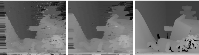
Fig. 1: Example of the Teddy dataset [8]. Left, right: RGB 1-D process without adaptive radius and grayscale 1-D process with adaptive radius without 2-D refinement. Right: Ground truth.
