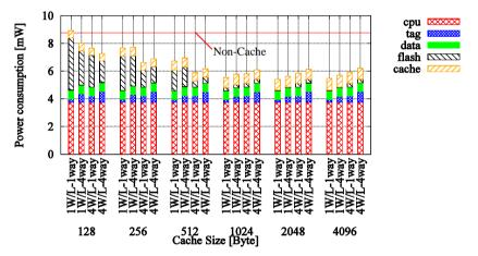
Figure 9. Power consumption by cache size. (Ratio of flash memory's power consumption: 50%)
