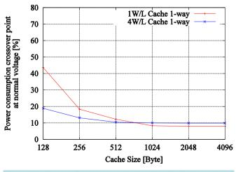
Figure 11. Change of crossover point by cache size for low-voltage operation.
