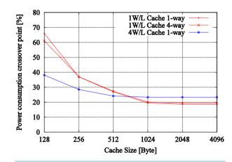
Figure 10. Change of crossover point by cache size for normal voltage operation.
