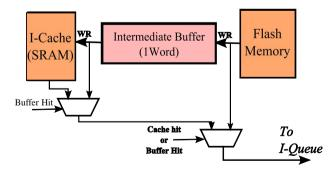
**Figure 3.** Intermediate buffer insertion method for 1-word-perline instruction cache architecture.
