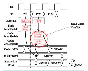
Figure 2. Instruction memory access timing in case of cache hit immediately after cache miss.
