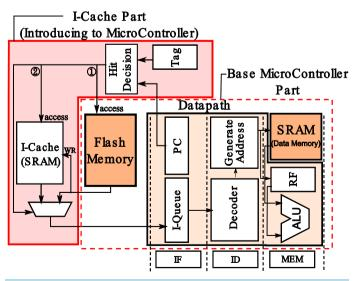
Figure 1. Concept of proposed 1-word-per-line instruction cache architecture.
